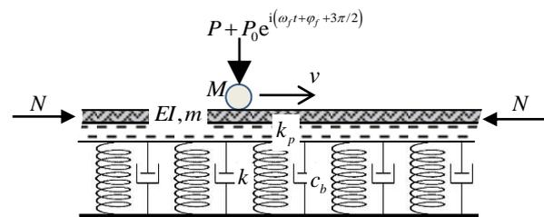
**Fig. 1.** Infinite beam on a visco-elastic two-parameter foundation subjected to a moving load and a normal force.
